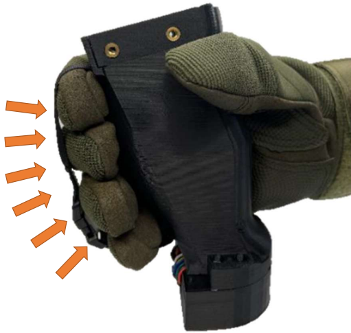
Figure 4: Haptic Feedback Device provides squeeze stimuli to the intermediate phalanges of the operator’s fingers to provide clear, unambiguous alerts of vehicle state.
